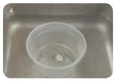
Clean restoration using an ultrasonic cleaner in alcohol or acetone, or steam cleaner
